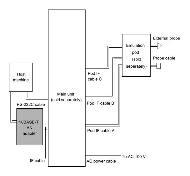
Figure 2.1 System configuration
